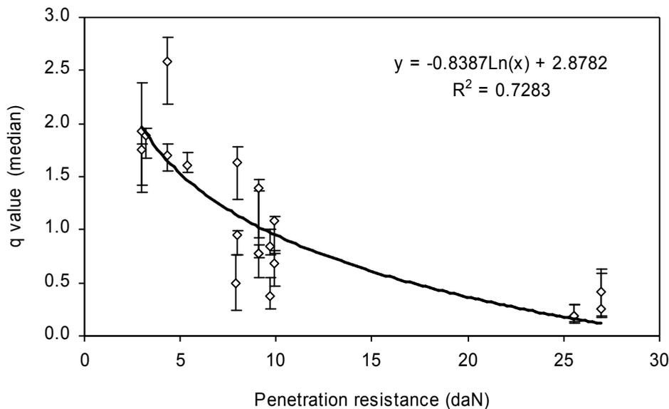
Fig. 2. q value (median) as a function of penetration resistance for mineral soils (Bastgen and Diserens. 2009)
