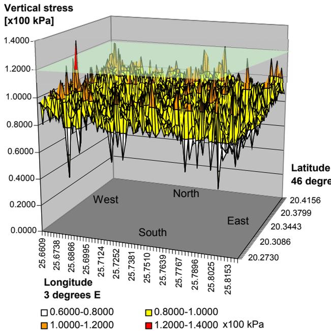
Fig. 5. 3D map of compaction damage risk. Vertical stress for a homogeneous firm soil with a stability point limit of 120 kPa for a loamy sand at 30 cm soil depth
