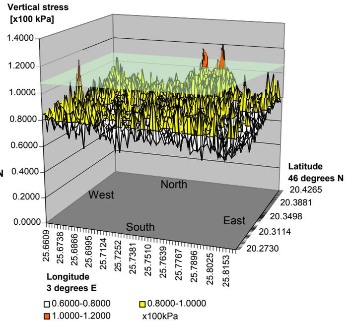
Fig. 6. 3D map of compaction damage risk. Vertical stress according to the distribution of penetration resistance values with a stability point limit of 108 kPa by 8.6% clay content at 30 cm soil depth
